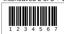
Interleaved 2 of 5 + CHECKSUM
